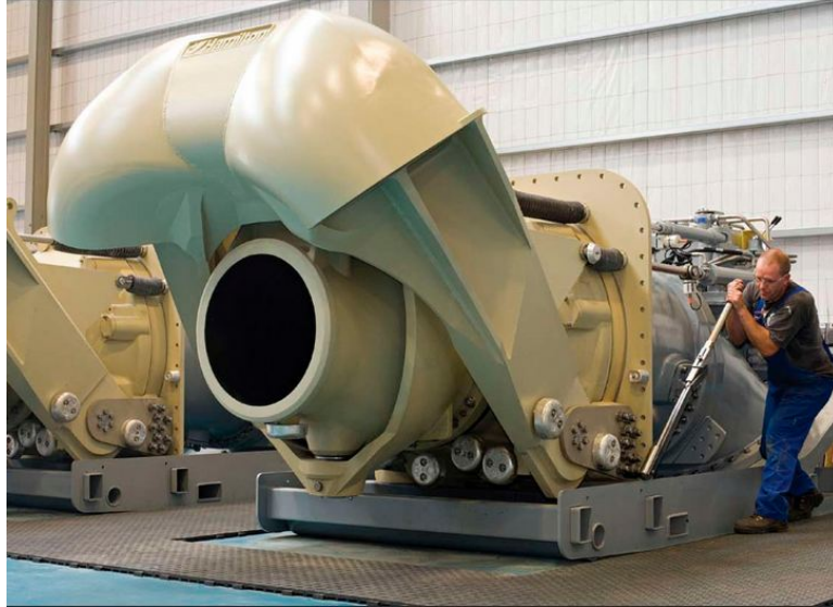
Figure 1.2: A water-jet propulsion system utilized for high-speed vessels (source: http://www.hamjet.co.nz/model_range ).
