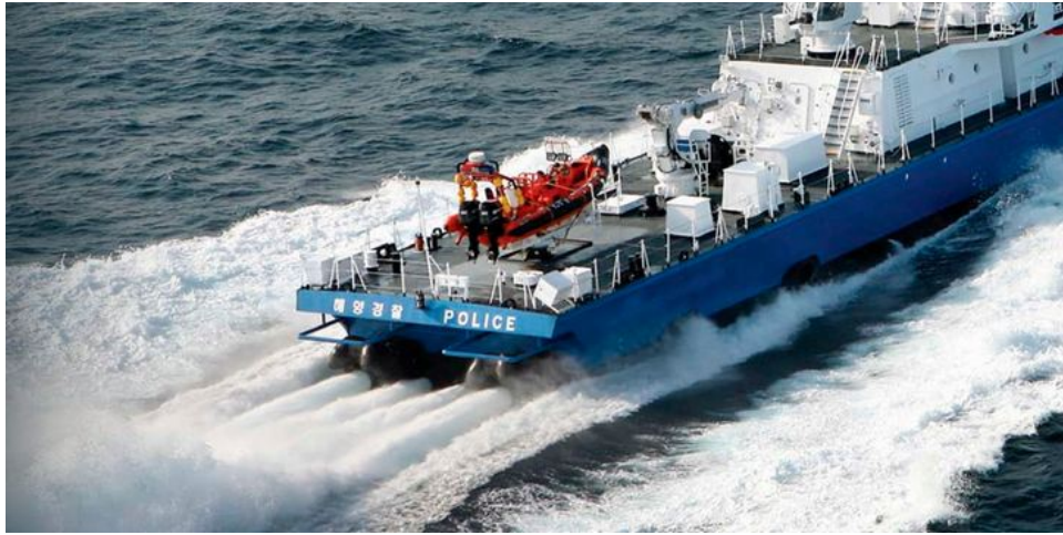
Figure 1.1: A high-speed police vessel utilizing water-jet propulsion (source: http://www.hamjet.co.nz/model_range ).
