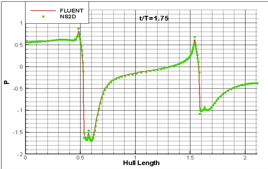
Figure 4.9: Pressure distributions along the fixed submerged hull subject to alternating inflow from NS2D and FLUENT at  $t/T_{in}=1.75$  ( $Re = 10^5$ ).
