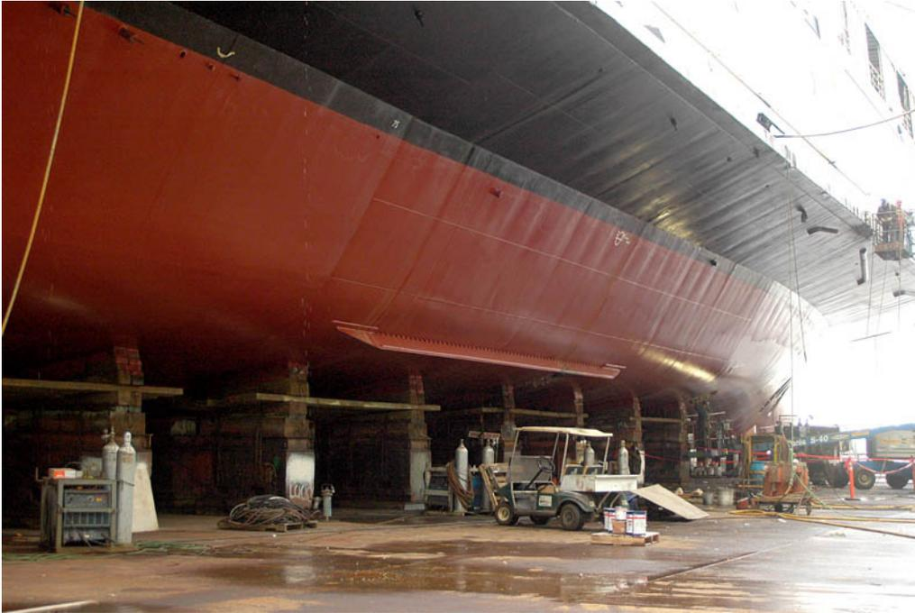
Figure 1.3: Mid-ship hull section showing bilge keels (source: [http://k43.pbase.com/v3/45/387545/1/50702675.DSC\\_3086z.jpg](http://k43.pbase.com/v3/45/387545/1/50702675.DSC_3086z.jpg))
