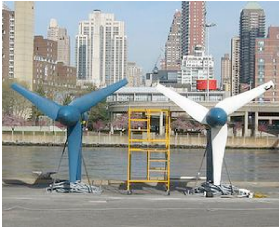
Fig 1.3 Two horizontal axis tidal turbines in New York's East River for Verdant Power's prototype tidal energy project (source: http://www.ens-newswire.com/ens/apr2009/20090409_tidalturbines.jpg )
