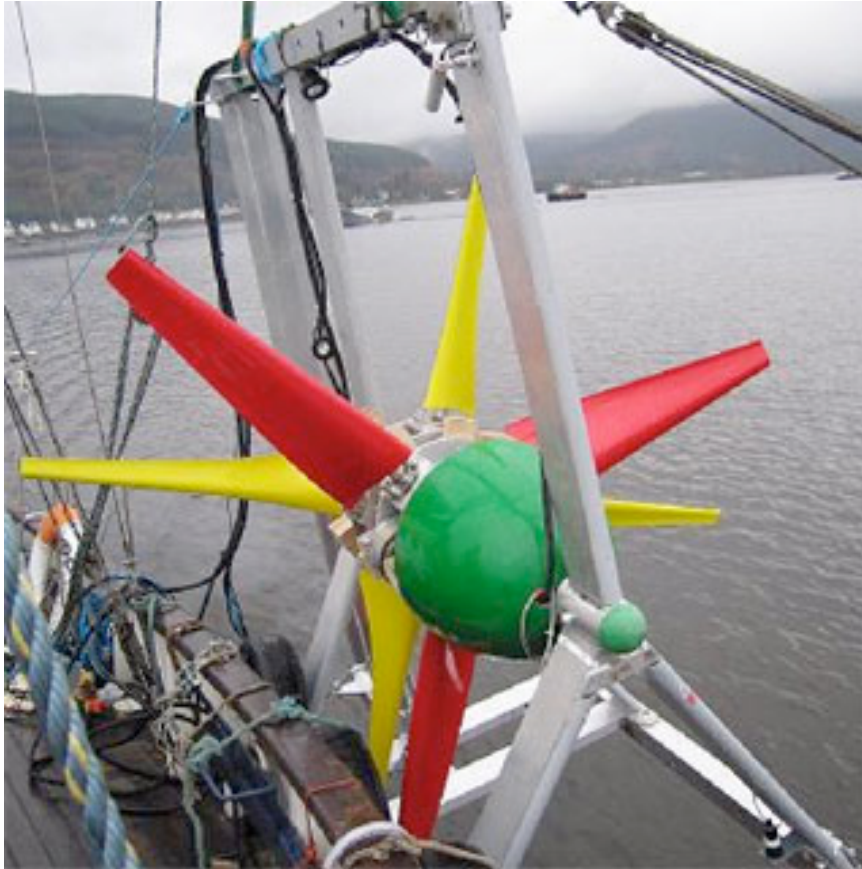
Fig. 1.5 2.5m diameter contra-rotating tidal turbine (Source: (Clarke, Connor, Grant, Johnstone, & Ordonez-Sanchez, 2008))
