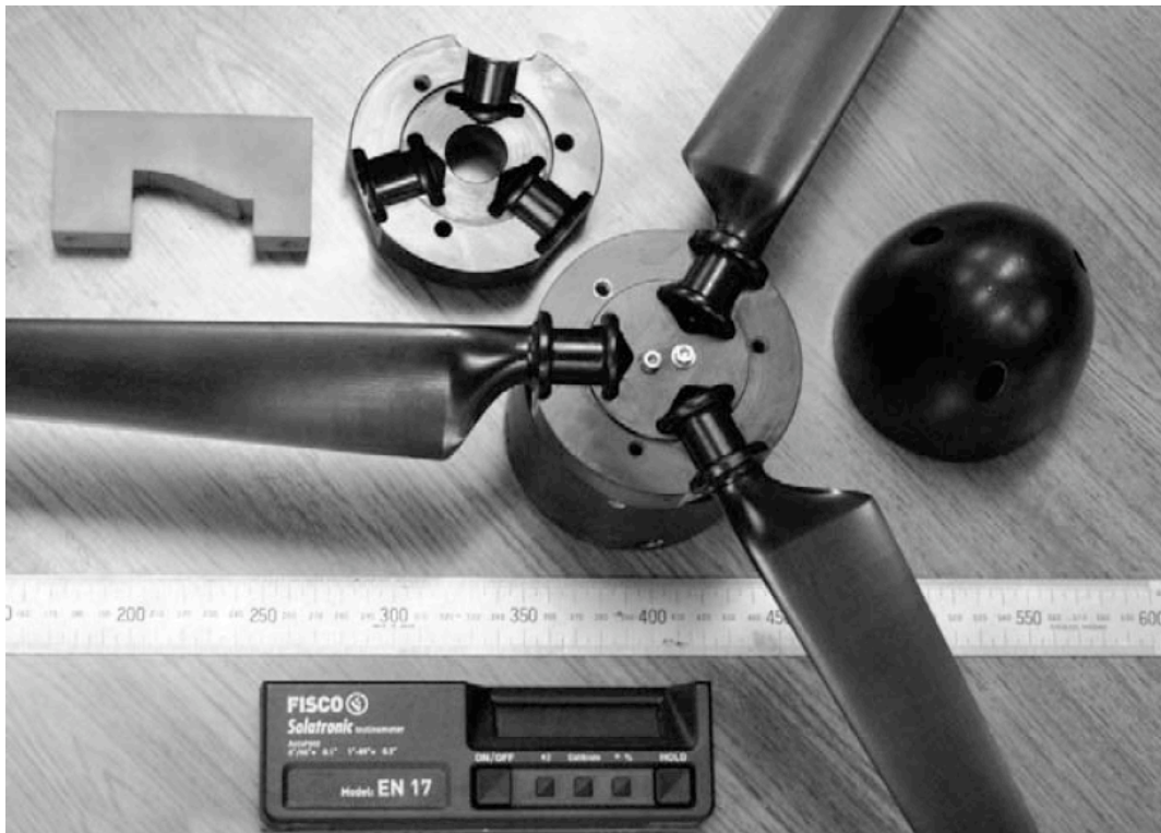
Fig. 4.11 Photograph of the blade and hub component (source: (Bahaj, Molland, et al., 2007))
