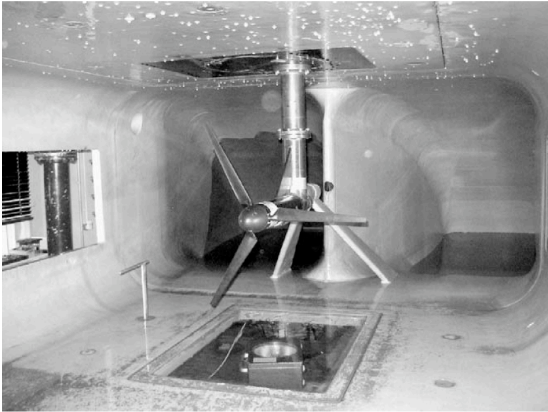
Fig. 4.10 Cavitation tunnel with a marine current turbine, from (Bahaj, Molland, et al., 2007).
