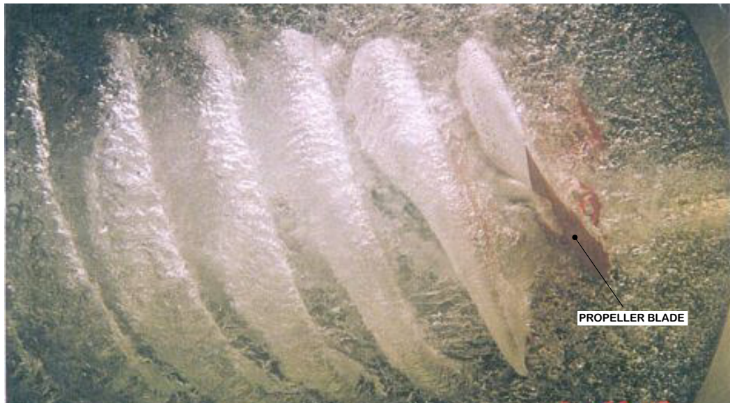
Figure 1.1: Ventilating cavities formed during the operation of a surface piercing propeller. View from underneath, with flow going from right to left. Taken from [Olofsson 1996].
