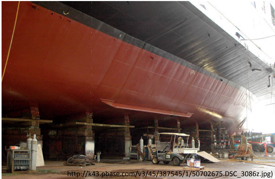
Figure 1.10: Typical hull with bilge keels
