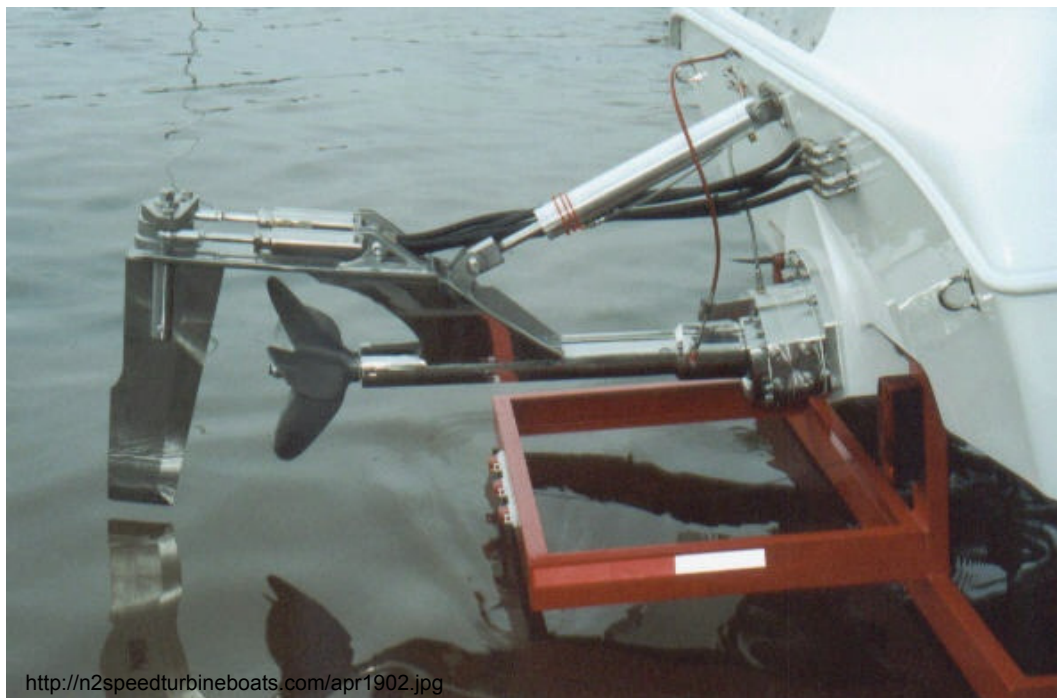
Figure 1.3: Typical surface-propeller drive arrangement
