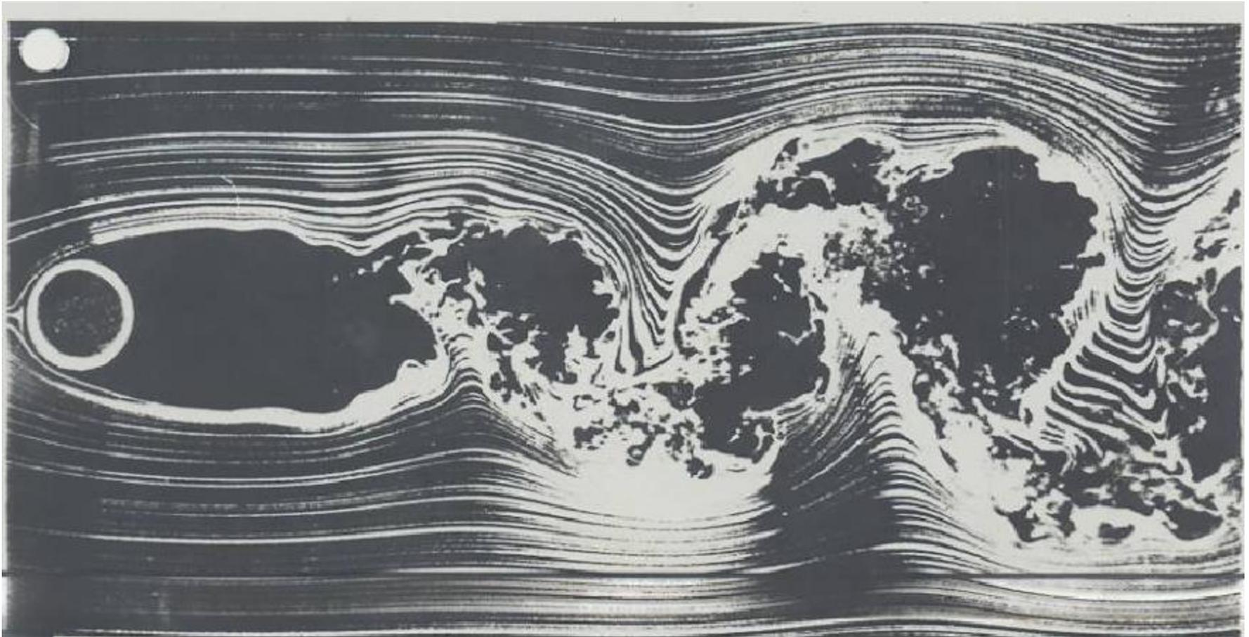
48. Circular cylinder at  $R=10,000$ . At five times the speed of the photograph at the top of the page, the flow pattern is scarcely changed. The drag coefficient consequently remains almost constant in the range of Reynolds
