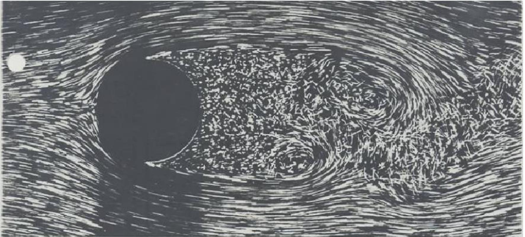
47. Circular cylinder at  $R=2000$ . At this Reynolds number one may properly speak of a boundary layer. It is laminar over the front, separates, and breaks up into a turbulent wake. The separation points, moving forward as
